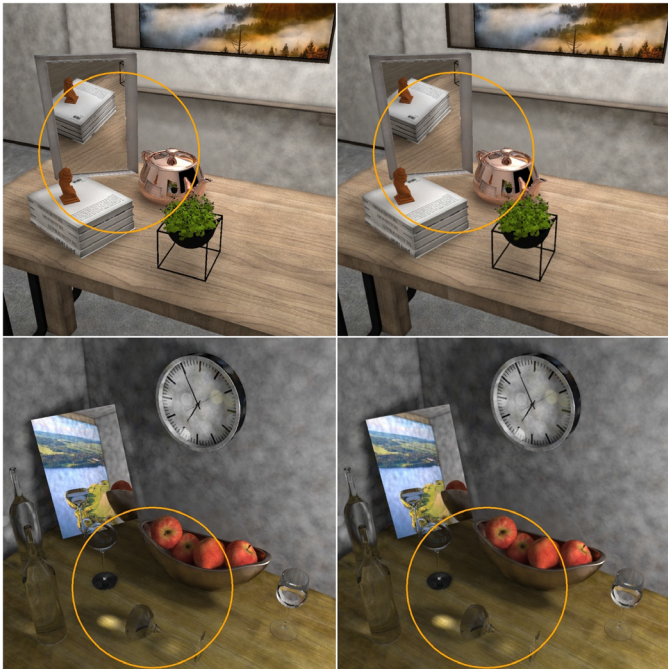
Fig. 8: The images rendered by using our method without (left) and with spatial filtering (right).
